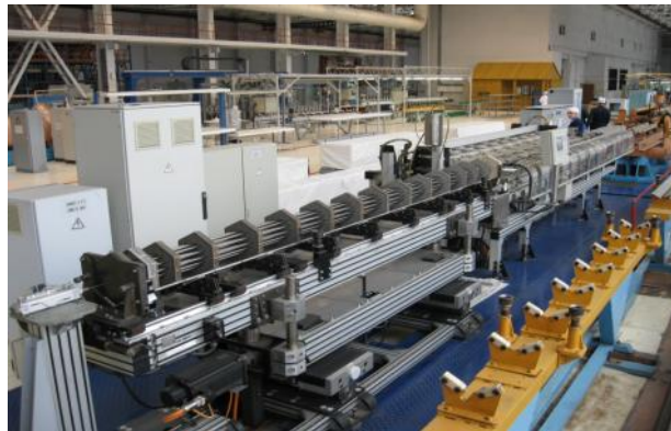
Automated bench for fuel bundle assembly
