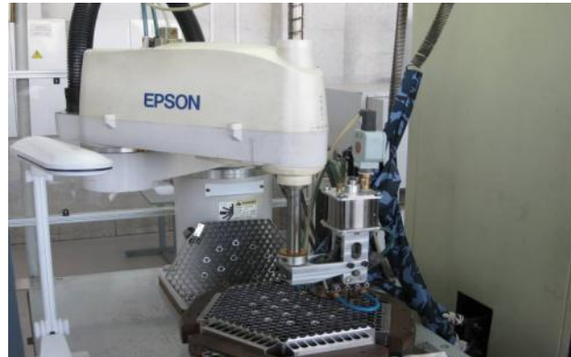
Robotized complex for spot welding of spacer grids
