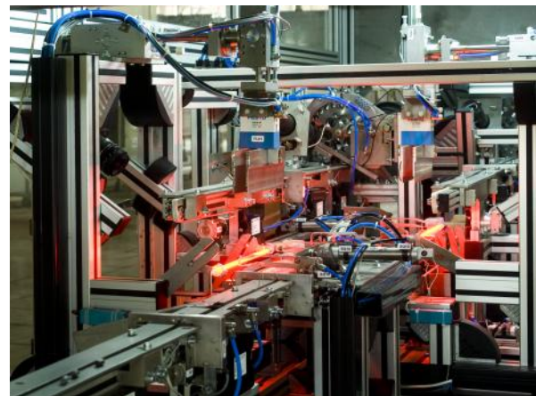
Equipment for optical inspection of pellets appearance
