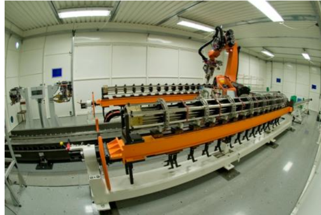
Robotized complex for assembly and welding of FA skeletons
