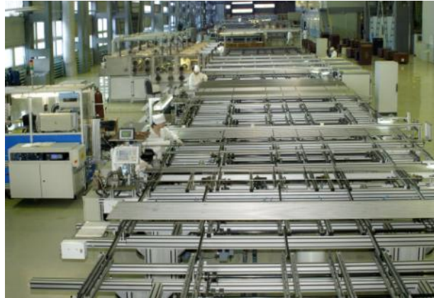
Line for fuel rod fabrication
