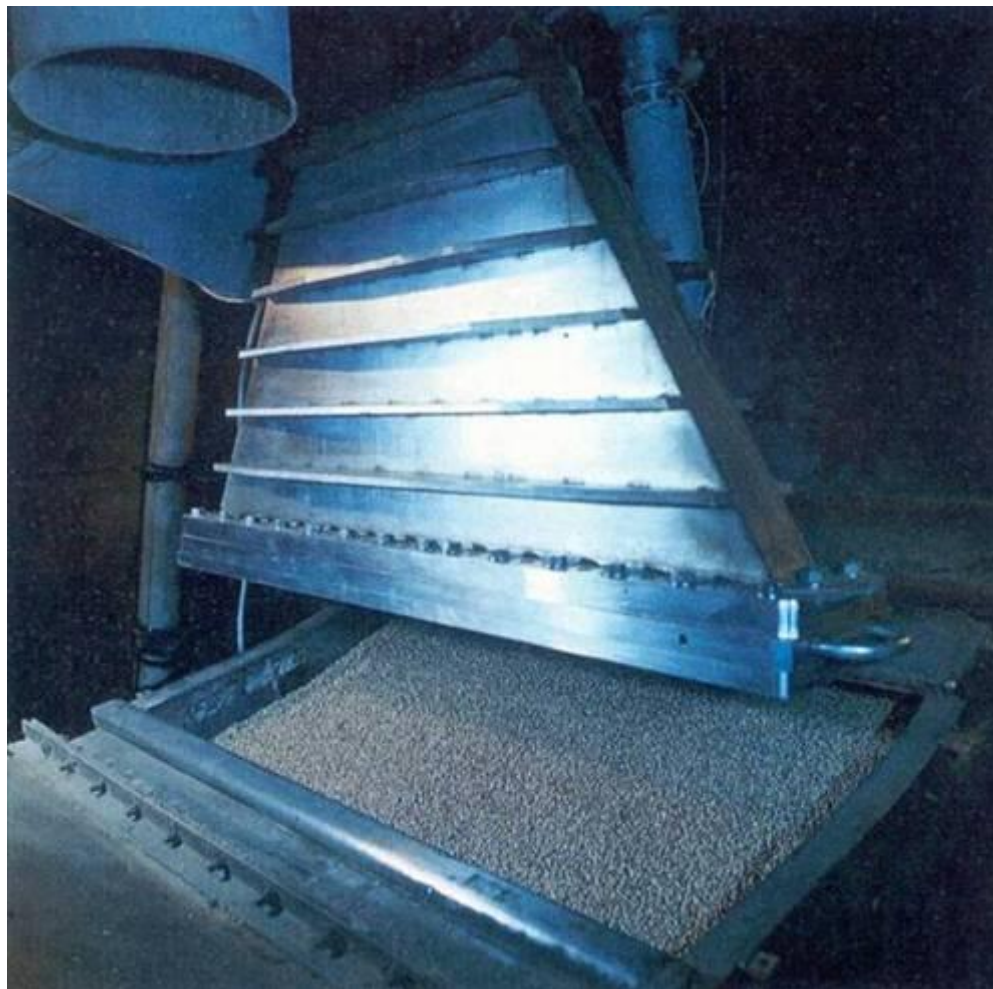
ELV-8 accelerator using for grain disinfestations with productivity of 1000 t/hour
