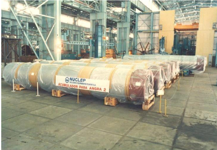
ACCUMULATORS FOR ANGRA 2
