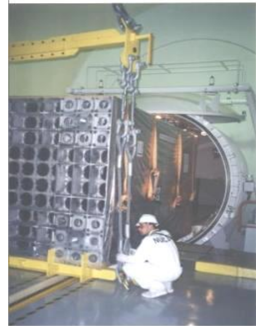
SUPERCOMPACT STORAGE RACKS FOR SPENT FUEL ELEMENTS FOR ANGRA 2
