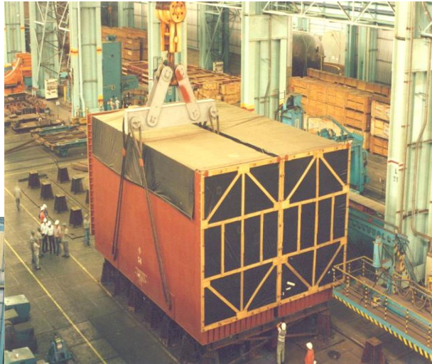
CONDENSERS FOR ANGRA 2
