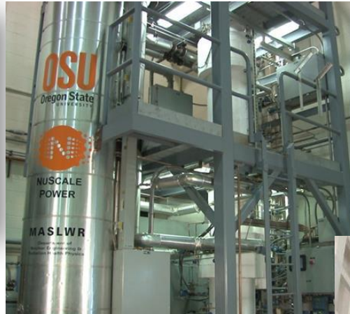
NuScale: NuScale Integral System Test (NIST) facility (1:1 in P, T; 1:3 in height, 1:253 in volume, 1:1 in time)
