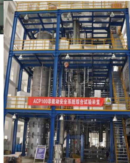
ACP100: Core Cooling and REsidual heat removal System Test facility (CREST) (1:1 in height and P, T; 1:37 in volume; 1:100 in power)
