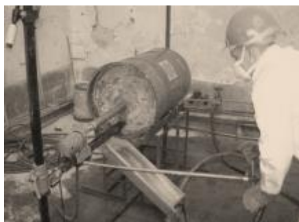
Sample collection of ceramics with and without sludge inclusions
