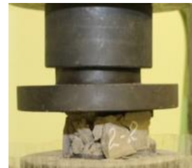
Mechanical tests of ceramics with sludge inclusions
