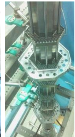
Mechanical testing of prototype and framework of peripheral zone FA and FA with CPS
