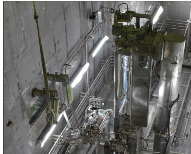
System for assembling fuel rods into the final fuel assembly structure
