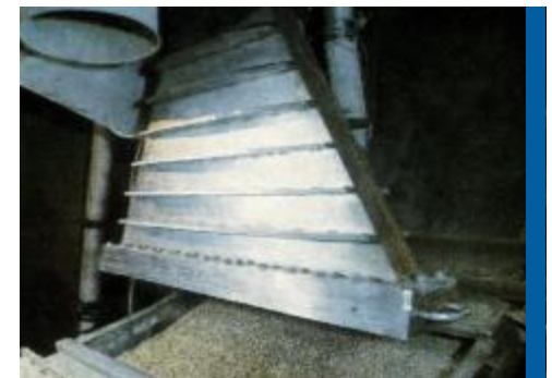
electron beam in the irradiation chamber for grain processing
