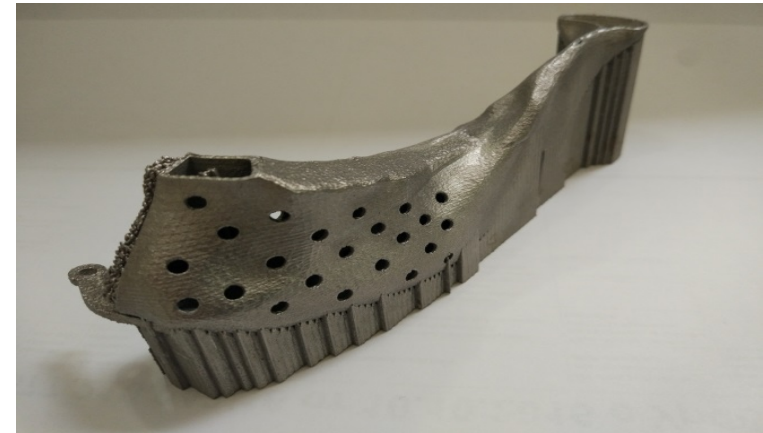
Segment of the lower jaw. The prototype of the implant is printed on a 3D printer MeltMaster3D-550 (CNIITMASH) made of titanium VT1-0
