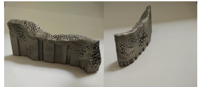
Segment of the lower jaw. The prototype of the implant is printed on a 3D printer MeltMaster3D-550 (CNIITMASH) made of titanium VT1-0
