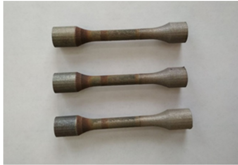
SLM directly printed samples
